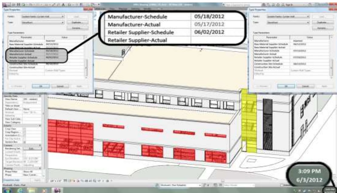
Figure 6: Generation of a 3D color-coded view of “material (e.g. curtain wall)” in the BIM model
