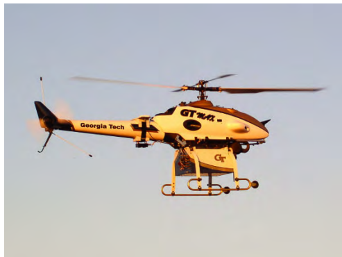
Figure 2. The GTMax helicopter weighs 66 kg and has a rotor diameter of 3 m. For vision-based navigation, a downward-facing camera is mounted on the nose of the vehicle.
