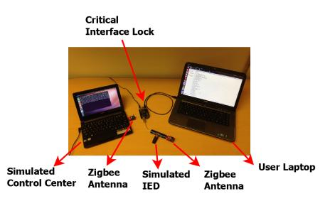
Figure 7: Current prototype being tested with USB flash drive and simulated control center.
