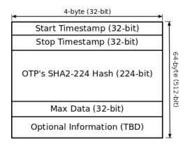
Figure 4: Maintenance Record Structure.
