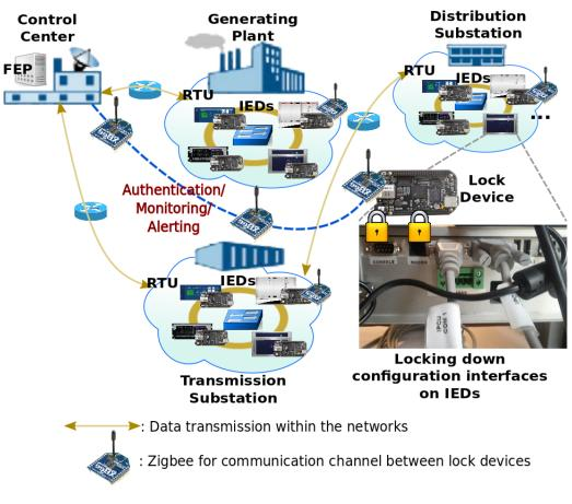
Figure 1: Deployment in Power System.
