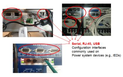
Figure 2: Variety of interfaces found on the back of an IED.
