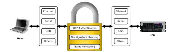
Figure 3: Modular design of CIL device.
