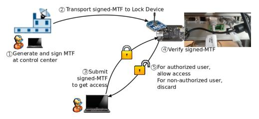
Figure 5: Procedure for loading a maintenance file (MTF) onto an IED.
