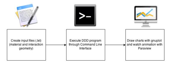
Figure 1 Workflow of executing the material-stress simulation
