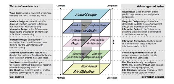
Figure 25 The elements of user interface [19]
