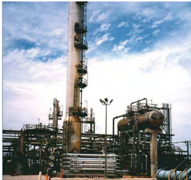
Figure 1.4: A skid-mounted membrane unit (in foreground) was installed to replace a bulky amine absorption process (in background) [8].
