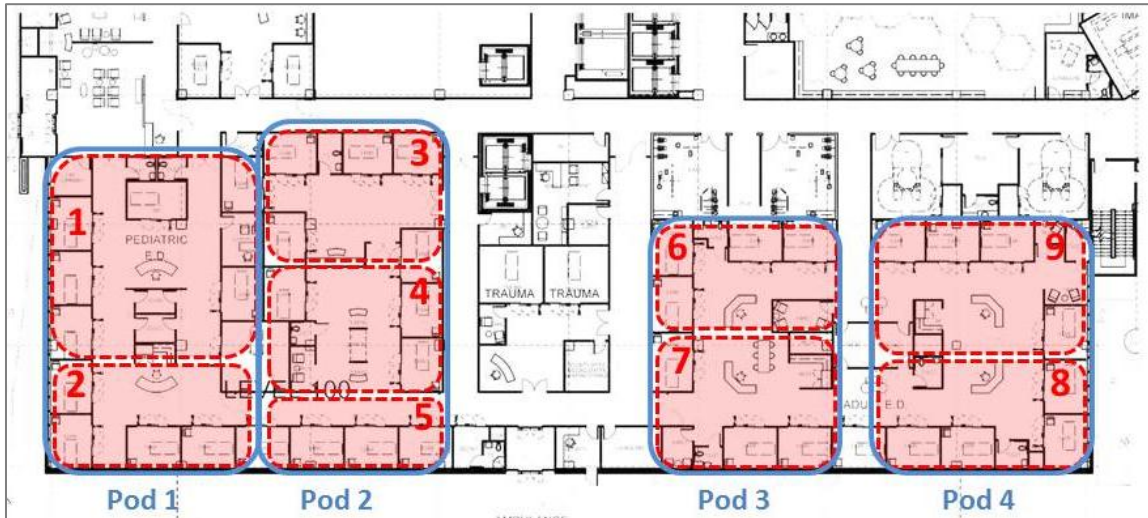
Figure 21. The layout of the ED based on 4 pods (in blue continuous line) consisted of clusters with four to five exam rooms (Markings by the author)
