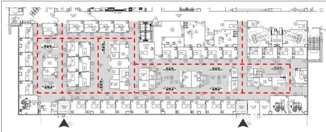
Figure 22. The revised ED layout with continuous corridors to enhance visibility and accessibility
