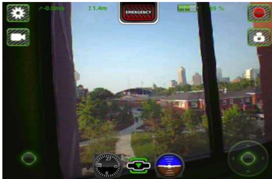
Figure 2-1: Example of UAV flight controller user interface – safety inspection experiment
