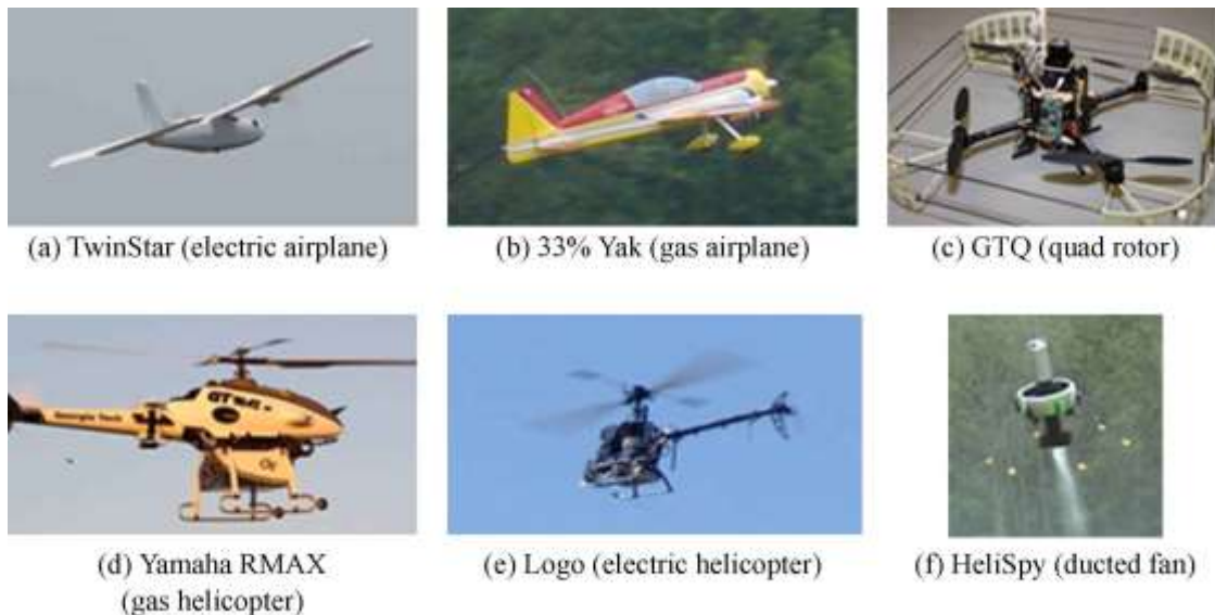
Figure 1-2: Some of the aircraft that have been utilized for research in the Georgia Tech UAV Research Facility, including a variety of configurations.
