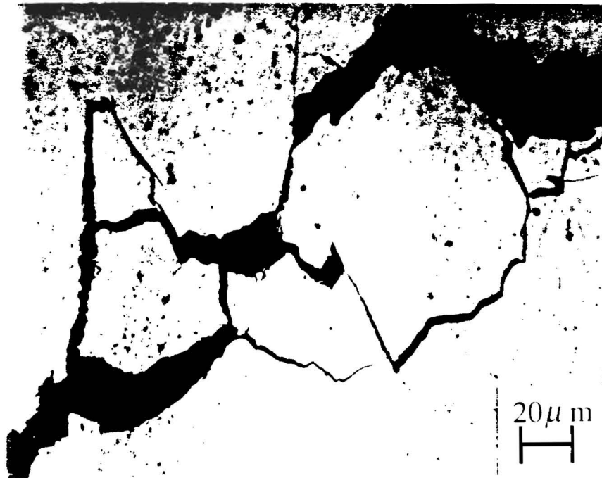
Figure 1.3: a) Opposite faces are "wedged open". b) Fracture surfaces are shattered and distorted due to contact each other.
