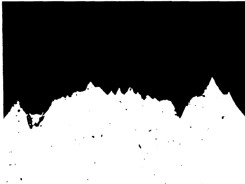
Figure 1.8: Digitization of crack profile of which dimensions are actual.
