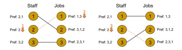
**Figure 4:** Example of the solution structure where Algorithm *minAgentNegotiations* has a worst case optimality gap of 100%.
