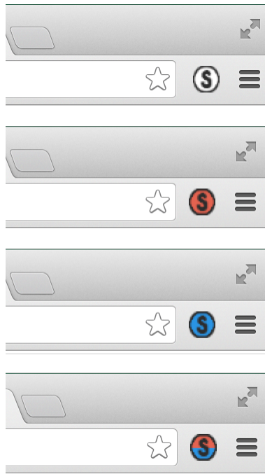
Figure 4: Button added to the user's Internet browser (here, Google Chrome) by Snack. A white background indicates the resource has not been saved to Snack while a red background indicates an EPHI advisor has saved this page (and notes) as a resource. Blue indicates the user has saved their own private notes on this resource (part of the enhanced version of Snack), and a red/blue icon indicates both public (advisor) and private (personal) notes are saved.
