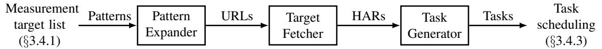
Figure 7: Encore transforms a list of URL patterns to a set of measurement tasks in three steps. A URL pattern denotes a set of URL ( e.g. , all URLs on a domain). A HAR is an HTTP Archive [80].
