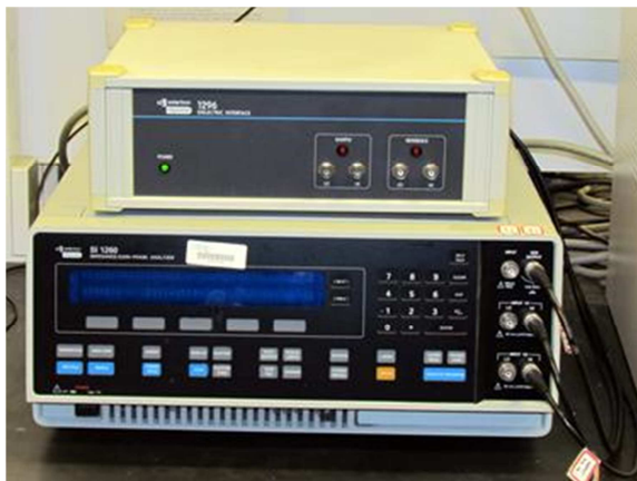
Fig. 3.6: Solartron 1260 attached to Solartron 1296 dielectric interface
