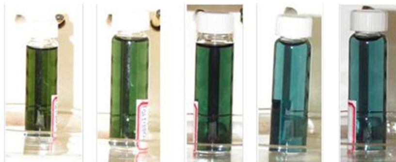
Fig. 4.3: ITO solution, and typical change of color with ageing
