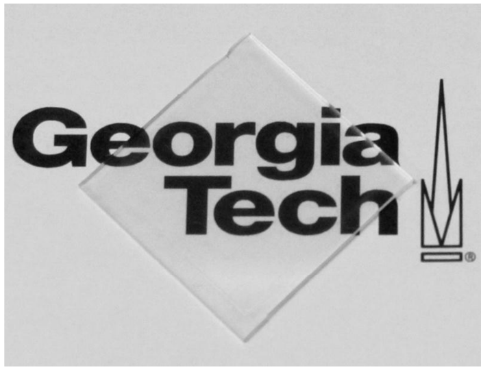
Fig. 4.7: As-spin coated colloidal ITO film on glass substrate
