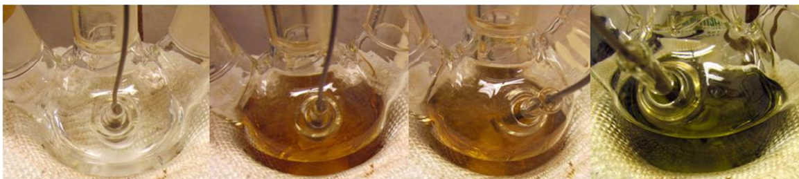
Fig. 4.1: Change in color of the solution during synthesis, going from colorless, shades of yellow, orange and brown to dark greenish-black
