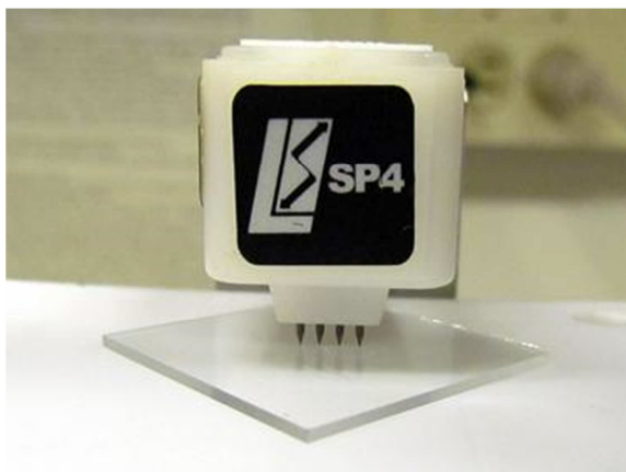
Fig. 3.7: Four point probe head being used for measurement on a coated substrate
