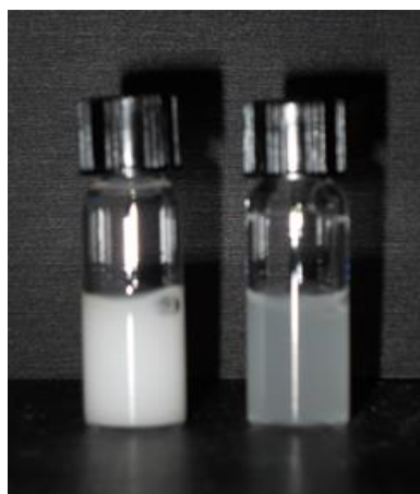
Figure 3.4. a) Images of vials containing pNIPMAM-BAC-BIS microgel dispersions (left) before and (right) after exposure to DTT.
