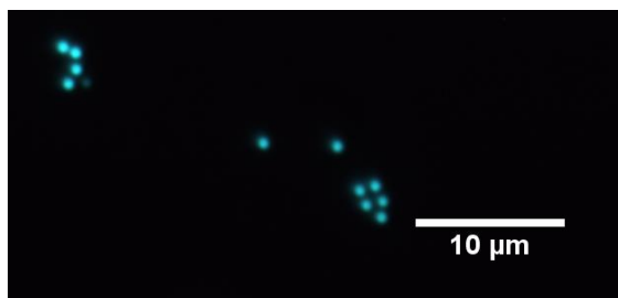
Figure 7.4. UV-excitation epifluorescence microscopy demonstrates that fluorescent labeling of pNIPMAm/2% BIS/2.5% BAC/10% AAc microgels with dansylcadaverine was successful. Scale bar is 10 \mu\text{m} .
