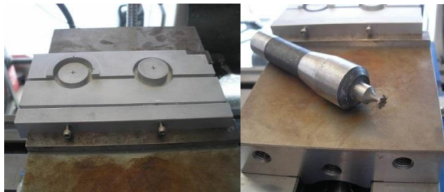
Figure G.5 | Jig used for cutting the O-ring grooves. Left: the jig is placed in the vise. Right: keyseat cutter used for cutting the grooves.
