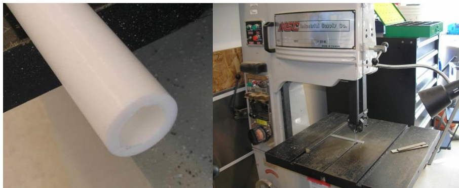
Figure G.1 | Teflon tubing is cut into 3/8 inch segments.
