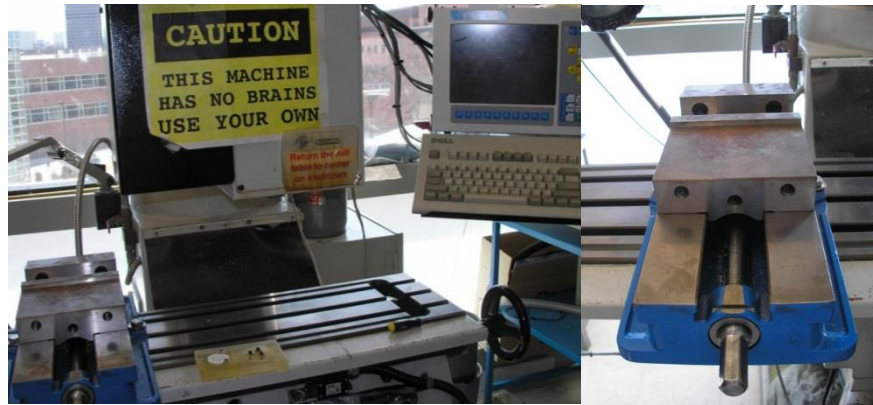
Figure G.2 | CNC Mill is used to cut lid diameters and O-ring slots.
