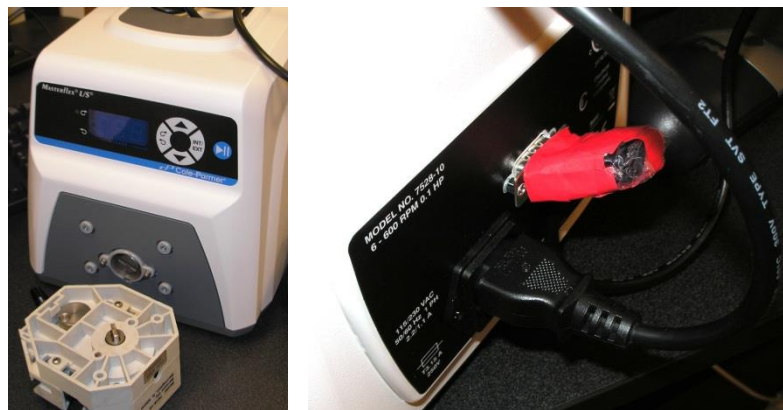
Figure D.5 | A modern digital Masterflex pump (model 7528-10) with reward circuit modification. Left: front of pump showing control panel and removed pump head. Right: Back of pump showing RS-232 + miniature low-signal relay modification (wrapped in protective red tape).
