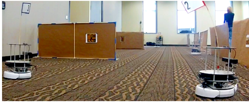
Fig. 11. Multiple robots are shown patrolling the museum environment from the viewpoint of a camera placed on robot 1. In this experiment, after robot 3 is observed performing poorly, its neighbors each pick up one of robot 3's tasks and send it a task reassignment message.
