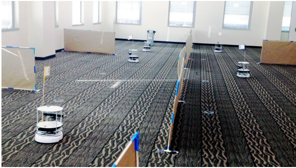
Fig. 4. Multiple TurtleBots are shown patrolling in the experimental environment, setup to resemble an art museum with multiple rooms.
