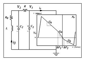
Figure 2: Chua's circuit diagram with nonlinear resistor  $N_r$
