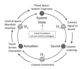
Figure 7: Schematic diagram of Playable Space of Chua's Circuit. The outer ring designates the physical system realization of the canonical inner ring structure.
