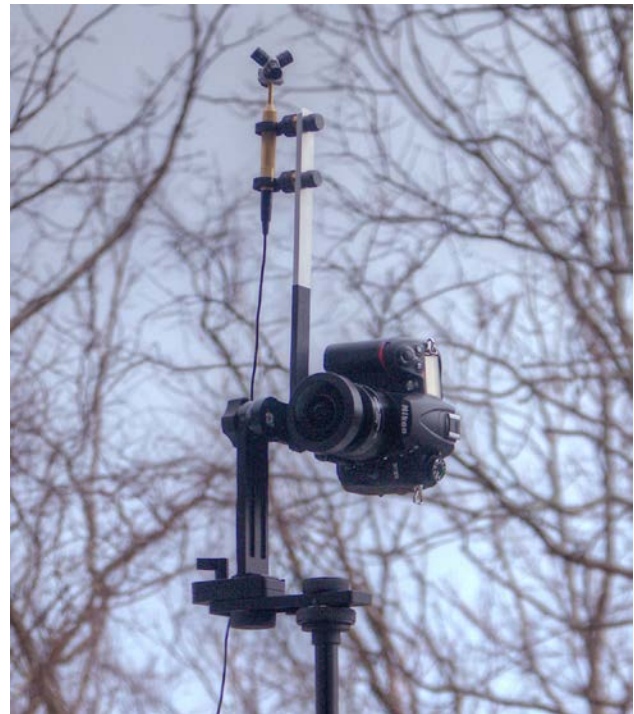
Figure 1: Image of author's cross-modal soundscape recording configuration comprised of Ambisonic audio capture and spherical panoramic photography.
