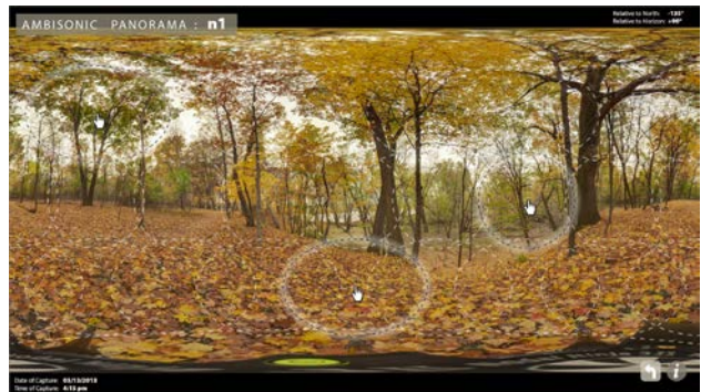
Figure 9: Example of a soundscape map from a single location, based on the equirectangular projection of a spherical panorama with embedded Ambisonic audio feeds, allowing comparison of directional sound arrival with visual context.
