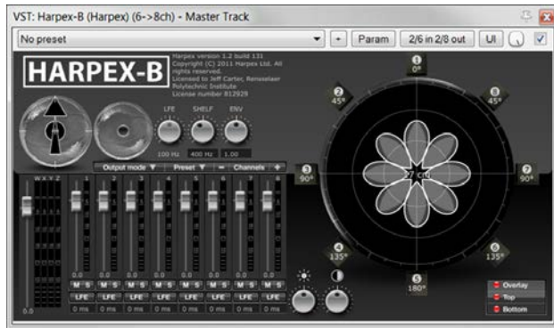
Figure 6: Screenshot of Svein Berge’s HARPEX-B format plug-in which is capable of deriving 8 virtual shotgun microphones per processing pass.
