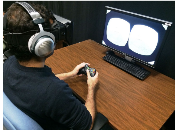
Figure 1: Directional source and spatial audio system integrated with Oculus Rift HMD and Half-Life 2 game engine.
