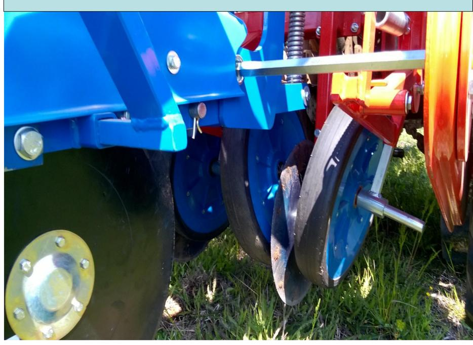
Figure 3. Double-disc openers for the furrow formation.
