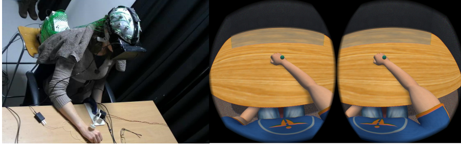
Figure 1. Experiment Setup. Left: Subject wearing the HMD, recording equipment and controller (under the desk). Mounted on the desk is the robotic actuator with the 3D printed ball attachment for delivering the tactile cue on the participant’s hand. Right: 2D representation of the visual stimulation from left and right eye view.
