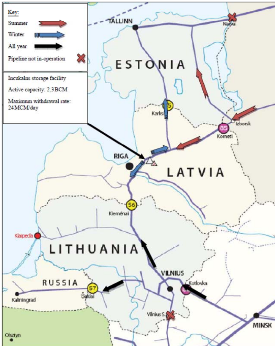
Figure 1 Baltic gas pipeline network
