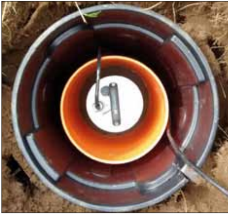
3 (Above) Seismometer installed in the ground at Sherbrooke Nova Scotia, part of the Maritimes QM-III deployment. (Amy Gilligan)
