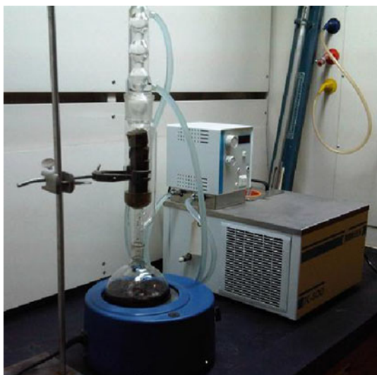
Fig. 5 Soxhlet apparatus containing some of the core samples used in this work
