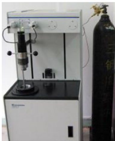
Fig. 3 Micro-Meritics automatic mercury intrusion apparatus (Auto-Pore IV)
