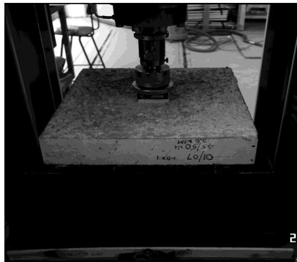
Figure 1 , Test set up for square panel
