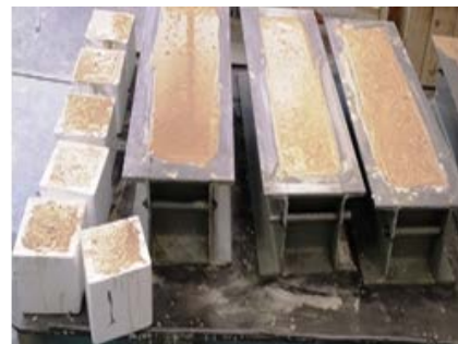
Figure 2. Fresh SFRC in beams and cubes moulds
