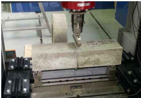
Figure 4. Three-point loading test of beam specimen
