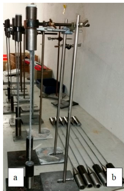
Figure 4. (a) Setup to cast epoxy grout anchorages; (b) Six CFRP specimens with testing anchors installed.
