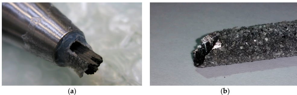
Figure 3. (a,b) Brittle failures of two UHM CFRP tendons at the load entrance of the resin-cast metallic barrel anchor used to anchor the tendons during the tensile tests.
