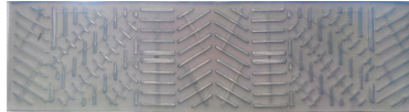
Fig. 4. Body wall of a body segment with Extensible Pneu-nets designed according to real muscle pattern on dissected and flattened body wall of Drosophila larva.
