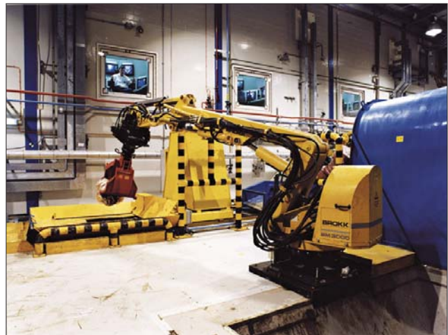
Fig. 1. A BROKK robot, equipped with a gripper, being used for a pick and place task at the Sellafield nuclear site in UK. This robot has no sensors for measuring joint angles, and so must be directly controlled by a human operator, who pushes a separate switch for each joint and judges the robot's pose by eye. The human operator can be seen controlling the robot from behind a 1.6m thick lead glass window which shields against radiation. For more examples, refer to www.sellafieldsites.com/solution/decommissioning/ .
