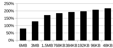
Fig. 18. Tag accesses for various tag cache sizes normalized to no tag cache
