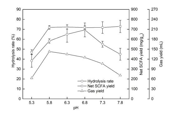
2 Fig. 2 – Hydrolysis rate, net SCFA yield, and gas yield at various constant pH values.
