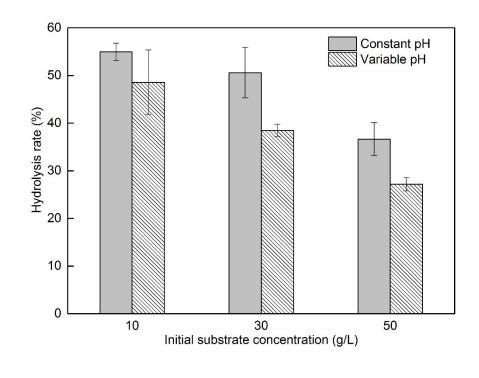
2 Fig. 4 – Hydrolysis rates of constant-pH and variable-pH samples in experiment C.
