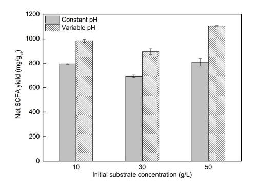
2 Fig. 5 – Net SCFA yield for the constant-pH and variable-pH samples in experiment
