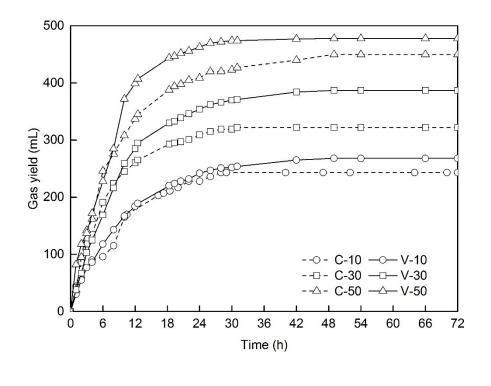
2 Fig. 6 – Gas yields of constant-pH and variable-pH samples in experiment C.
