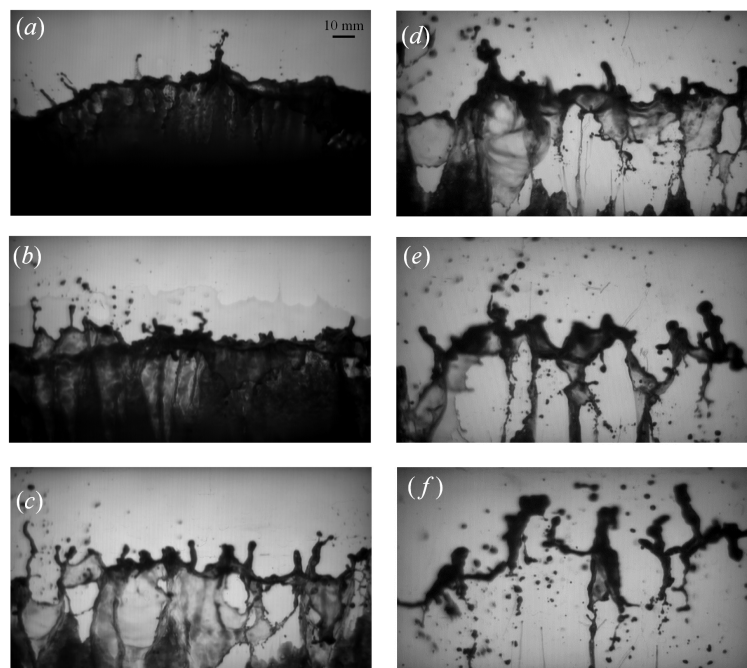
Figure 7. Evolution of transverse surface forms of the flip-through jet via fingering, rupturing film and breakup into sprays; (a) to (f) represent the vertical level z = 50, 100, 150, 200, 250, 300 mm.
