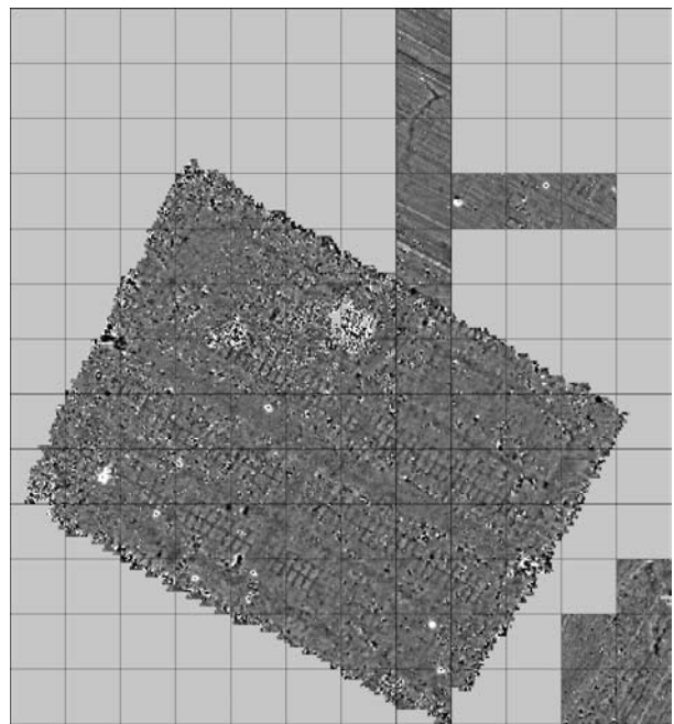
Fig. 3. Magnetometer Survey of Fort 4 on the Gorgān Wall by the joint project, Abingdon Archaeological Geophysics and the ICHHTO, notably Roger Ainslie et al., showing clearly three of the fort's four double barracks. Each survey square measures 30 x 30 m
