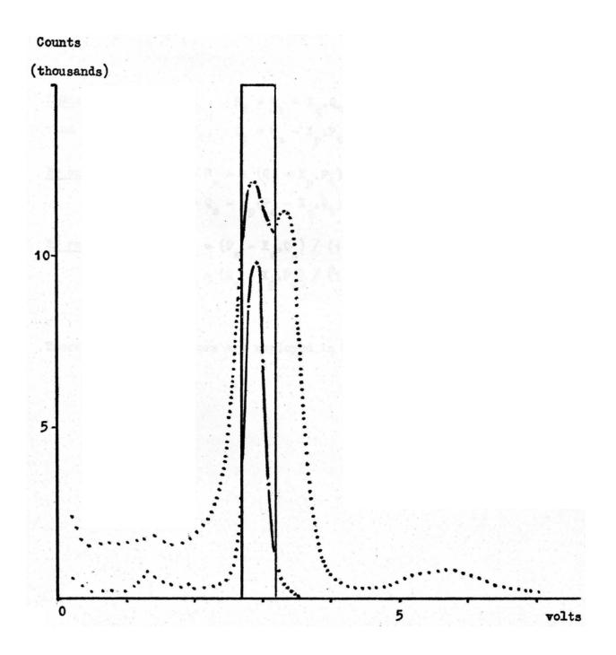
12. Correction factors for cross over in a two-isotope mixture
