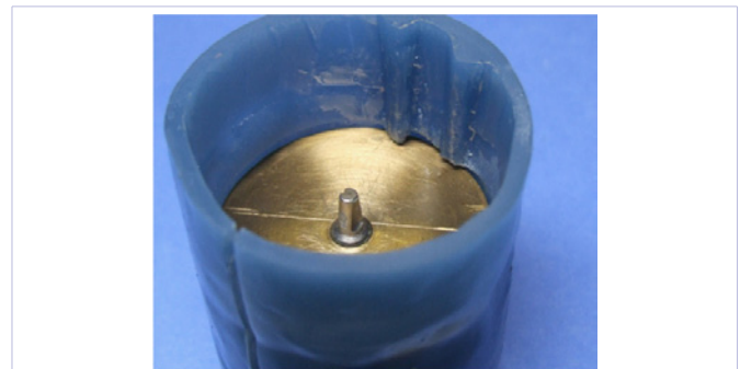
Figure 1c: Cylinder from light cured composite tray material made to fit accurately around brass casting which included 2 lugs on its internal surface.
