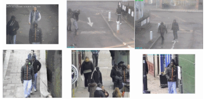
Fig. 1. Variation in low-quality CCTV images with poor lighting and long range camera views. Images taken from the same camera at different zoom levels. When a subject appears in the distance, the color and texture definition is poor and inconsistent with frames when the subject is closer.
