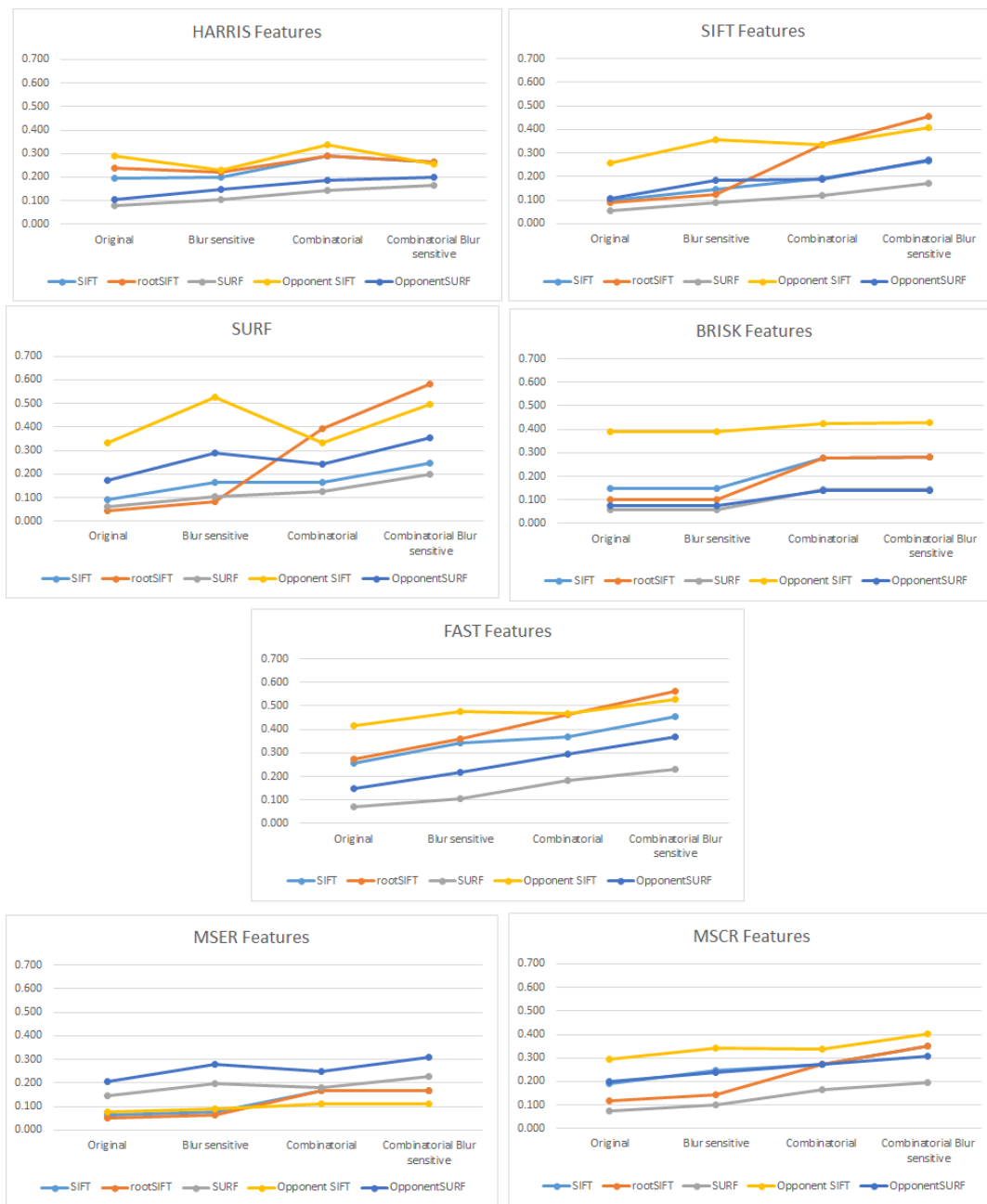
Fig. 16. Summary of the results of feature matching with each component of our method, and the combined methodology (right-most). Each graph shows results from a different feature detector, and compares results with each of four intensity and color descriptors using four methods; original – using Euclidean distance of unmodified feature descriptors is the baseline against which we measure performance improvements, Blur sensitive – blur sensitive feature detection algorithm using unmodified feature descriptors, Combinatorial – combinatorial texture and color feature matching descriptor extensions and matching algorithm, Combinatorial Blur sensitive – the combined methodology described in this paper.
