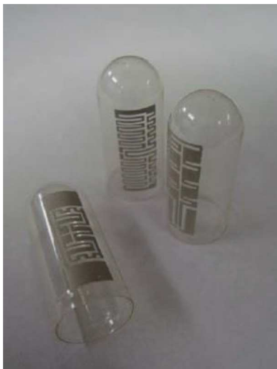
Figure 3.3: Bio-compatible capsule with embedded antenna (reproduced from [26])
