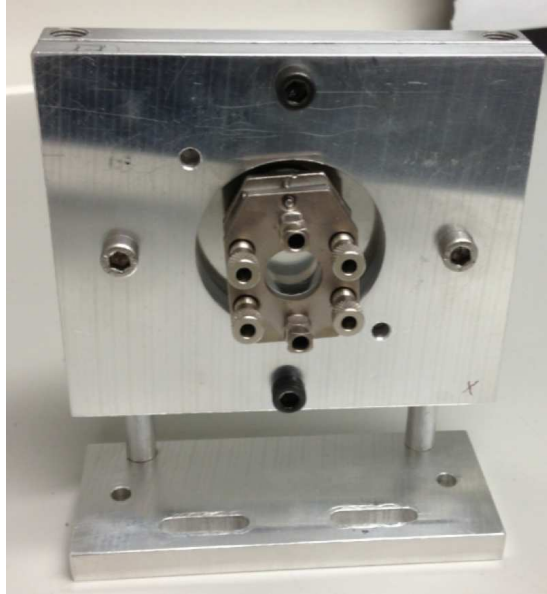
Figure 6.3: Sample holder with the stand
