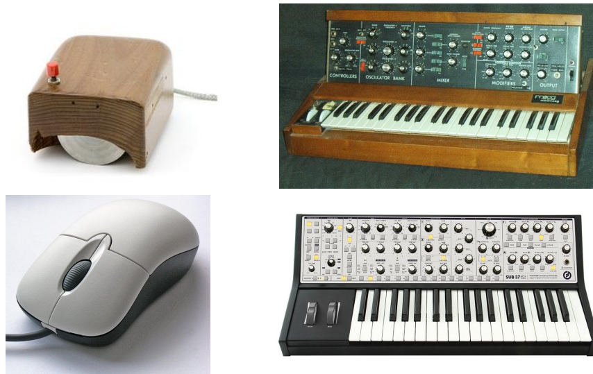
Figure 1.1: Fifty years of interface research has not resulted in many revolutionary designs reaching the mainstream, though perhaps a tendency to construct devices from plastic instead of wood. Top left: Douglas Engelbart’s mouse [English et al., 1967]. Bottom left: a modern mouse (2014). Top right: the Minimoog (1970)[Pinch, 2003]. Bottom right: the Moog Sub 37 (2014).
