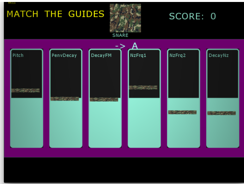
Figure 8.3: Slider interface for 6-DOF performance. Visual target settings (“guides”) appear as textured bars on the slider. Similarly to Experiment 2, a tap anywhere along the slider would set the bar to that location.
