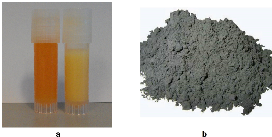
Figure 3.1: Ge QDs product ( a left) in original chemical solution and in ( a right) ethanol after being extracted from the original chemical solution. ( b ) Bulk Ge powder [188].
