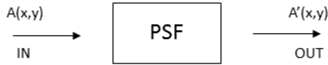
Figure 1.9: Image formation of microscope in the view of signal processing.
