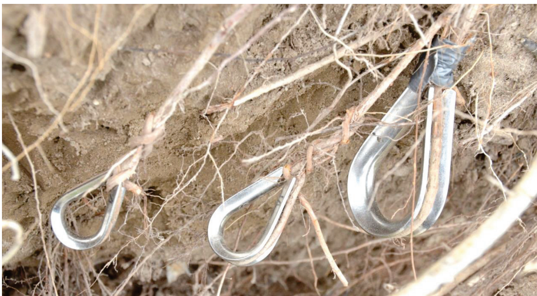
Figure 7.4 Use of rigging thimbles for applying load to roots more evenly.
