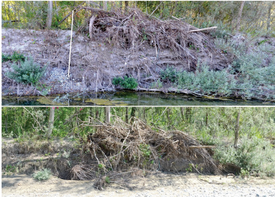
Figure 4.4 Site 5 during root and sediment sampling in 2013 (top) and during validation sediment sampling in 2014 (bottom) showing aggradation of the side channel bed between 2013 and 2014. Measuring staff visible is 3 m.
