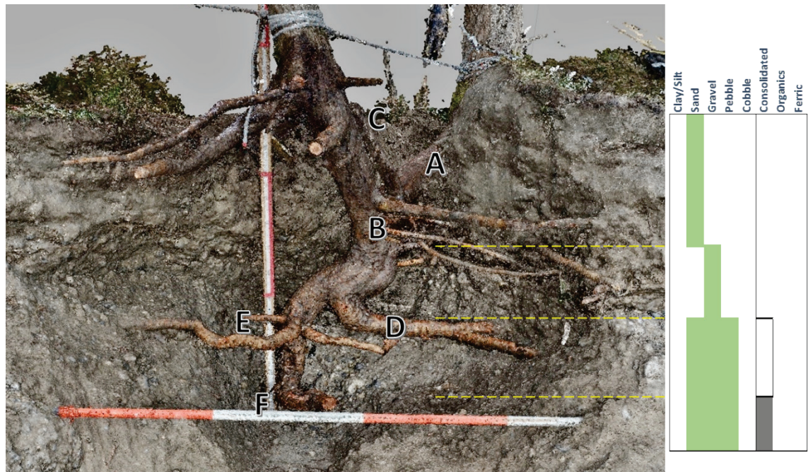
Figure 6.45 Front perspective view of RE model with key features and main sedimentary strata identified. The image has been mirrored such that flow is left to right. See further explanation below and in the introduction to this Section.
