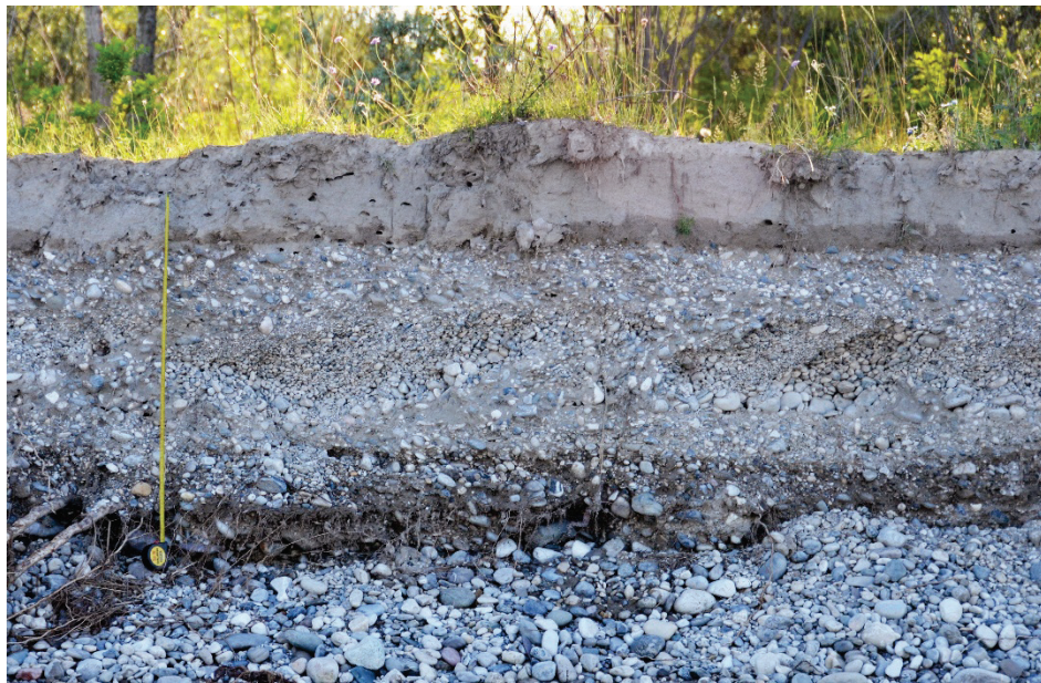
Figure 5.1 An example of the diverse, layered and patchy sediment types found in riparian soil profiles on the river Tagliamento. Tape measure at left is extended to 1 m.
