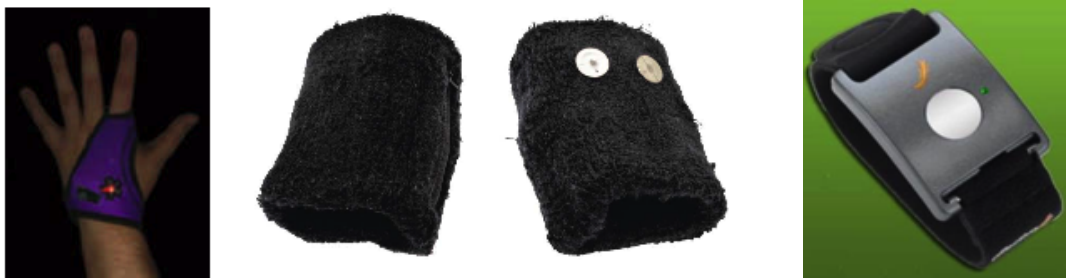
Figure 4.4: Picard's Galvactinator's progressive transition to the Q sensor (left to right)
