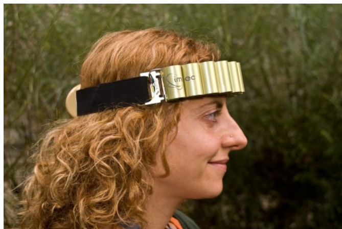
Figure 4.8. Imec's thermal powered EEG headset 21 .
