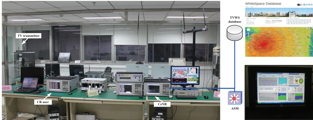
Fig. 6: CR enabled TD-LTE Test-bed.
