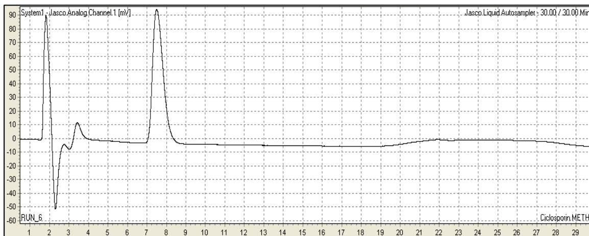
Figure 3.4: Chromatogram showing ciclosporin standard, column temperature at 75 °C
