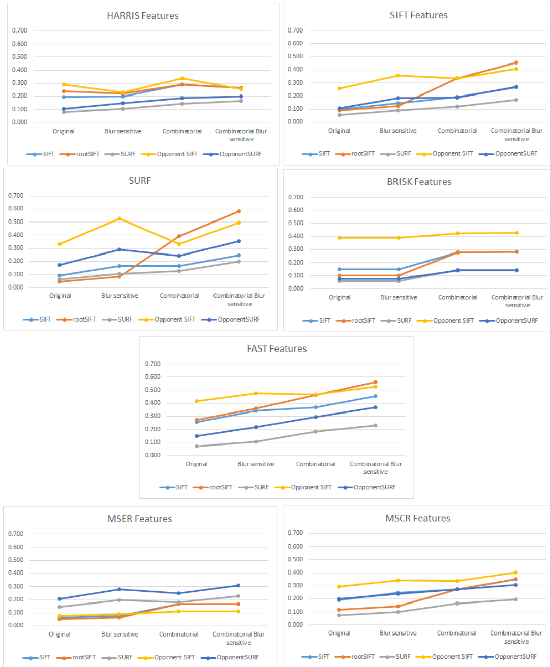
Fig. 9: Summary of the results of feature matching with each component of our method, and the combined methodology (right-most). Each graph shows results from a different feature detector, and compares results with each of four intensity and colour descriptors using four methods; original – using Euclidean distance of unmodified feature descriptors is the baseline against which we measure performance improvements, Blur sensitive – blur sensitive feature detection algorithm using unmodified feature descriptors, Combinatorial – combinatorial texture and colour feature matching descriptor extensions and matching algorithm, Combinatorial Blur sensitive – the combined methodology described in this paper.
