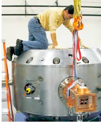
Figure 3.1: The Monarch 250 Cyclotron is an example of a compact (250 MeV) superconducting cyclotron which can run at 10 T and which uses the technique of resonant self-extraction. This was designed at MIT for proton therapy applications.
