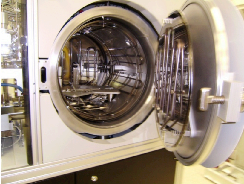
Figure 17: The Beneq ALD reactor purchased for Incom’s MCP fabrication facility.
