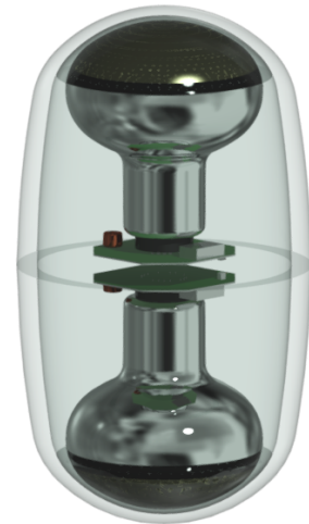
Figure 1: The shape of D-Egg. The height of the glass is 534 mm and the diameter at the equator is 300 mm.
