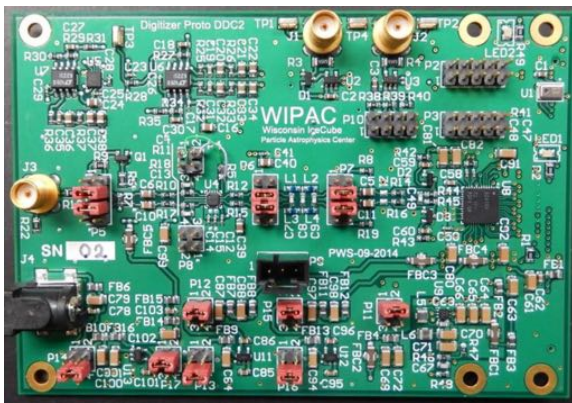
Figure 3: The prototype Digitizer Daughter Card (DDC2).
