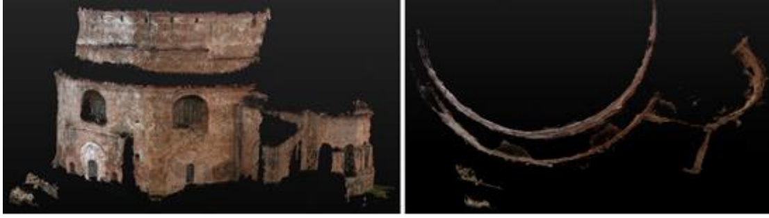
Figure 45. Rotunda 3D Reconstruction
