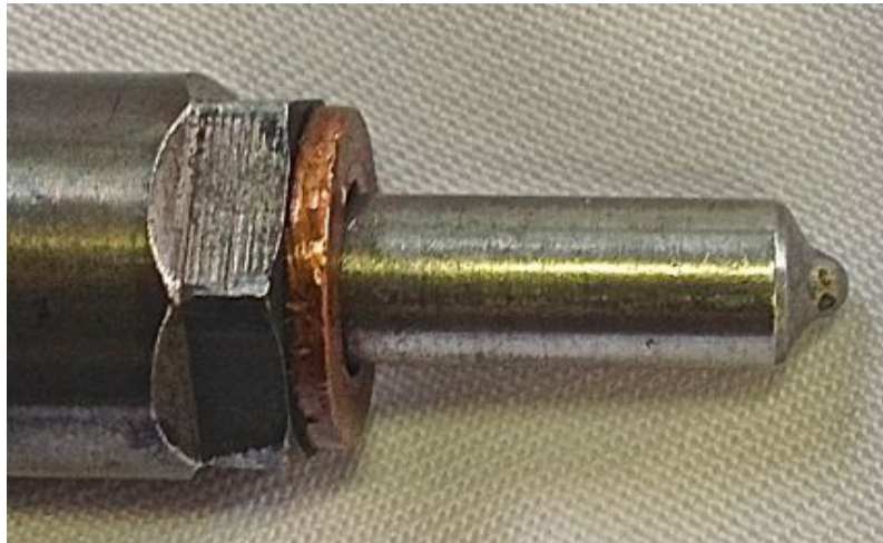
Figure 3.4: Photograph of the modified injector nozzle. The holes that have been welded are visible on the tip as small black dots.
