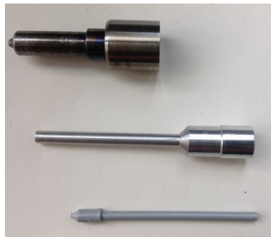
Figure 3.2: Photograph of the injector nozzle tip (top), the aluminum tube used to fill and extract the silicone from the nozzle (middle) and an example silicone mold (bottom).
