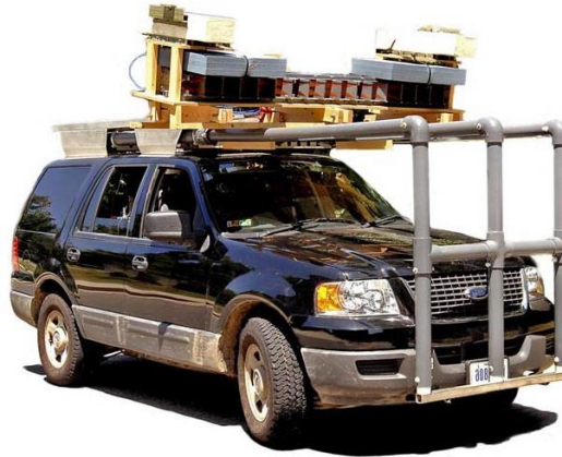
Figure 2-16 The ARL UWB SIRE radar system integrated onto the vehicle [72].
