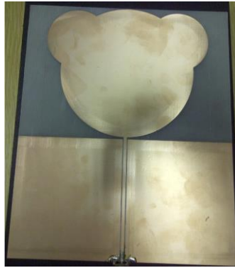
Figure 2-15 The Mickey Mouse monopole antenna developed in University of Liverpool [67].
