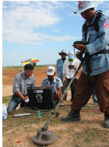
Figure 2-10 ALIS system with the cavity spiral antenna [56]
