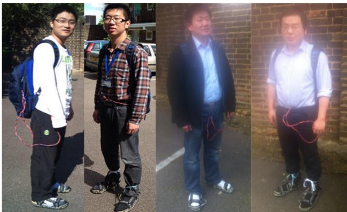
Figure 4.8: Participants with the First Prototype (that used a Phidget device, laptop and Smart Phone) During Mobility Data Collection
